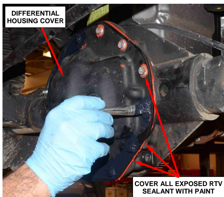
Figure 13 – Apply Black Paint to Exposed RTV Sealant
