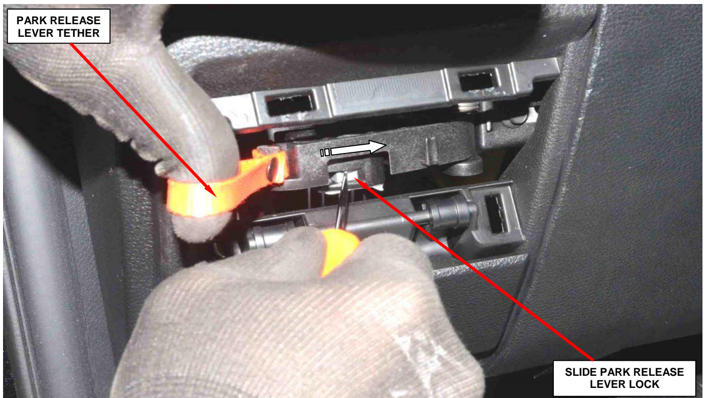
Figure 2 – Transmission Manual Park Release
