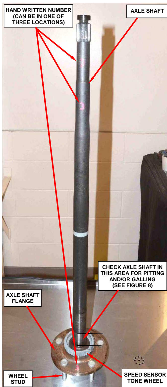
Figure 7 – Inspect Hand Written Number on Axle Shaft
