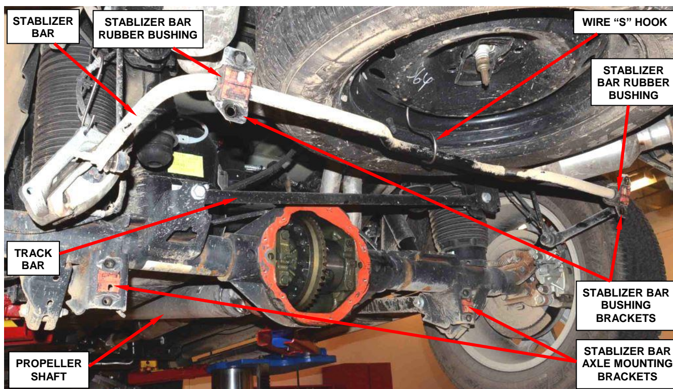
Figure 9 – Relocate Stabilizer Bar to Gain Clearance to Install Rear Axle Cover
