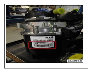
• Identify the part number on the label attached to the power steering pump
