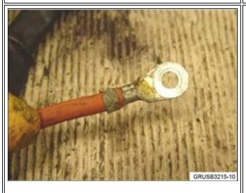
Ground connection without protective heat shrink tubing around cable eye crimp.
