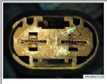
Connector with corrosion
