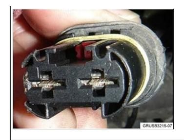
Connector without corrosion
