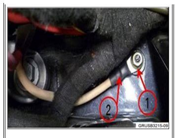
engine support with heat shrink tubing (2).
