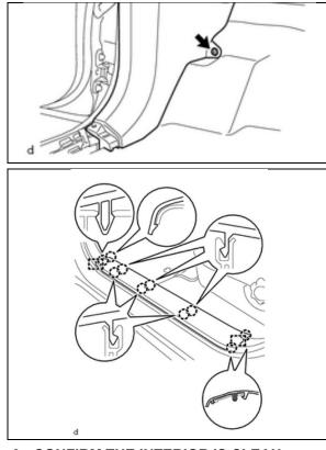
c) Install the clip onto the floor stud.
