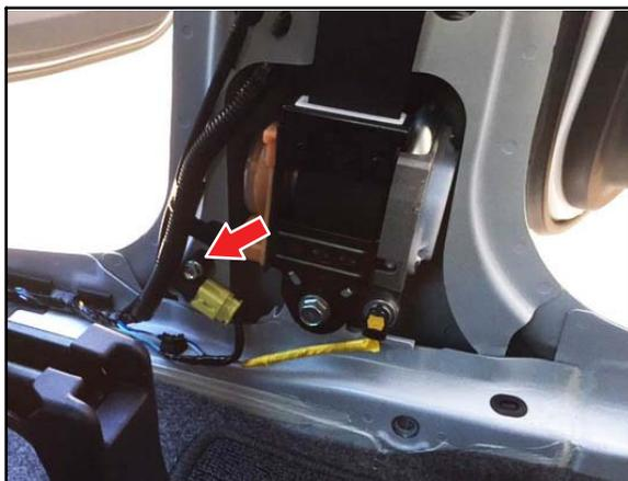
3. Remove the fitting nut for the side impact sensor.
