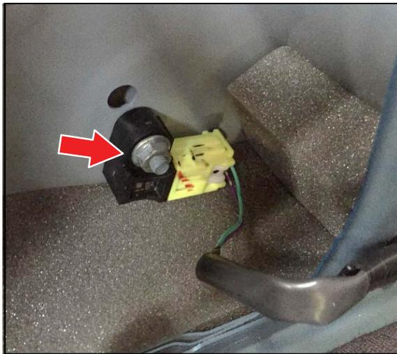
6. Remove the fitting nut of the side impact sensor.
