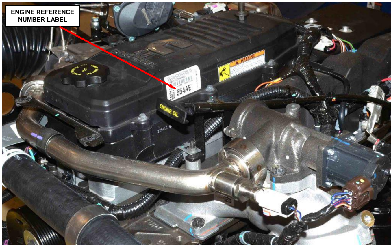
Figure 3 – Engine Reference Number Location (engine beauty cover removed for photographic purposes only)
