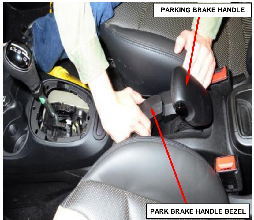
Figure 2 – Park Brake Handle Bezel
