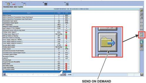
2. Update the A/T software with the MVCI. Refer to Service Bulletin 01-023, *Updating Control Units/Modules*. END
