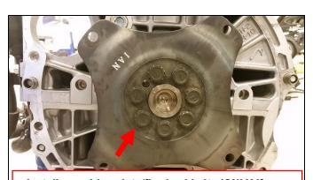
Install new drive plate/flywheel bolts (ONLY if new bolts are included with the replacement engine)
