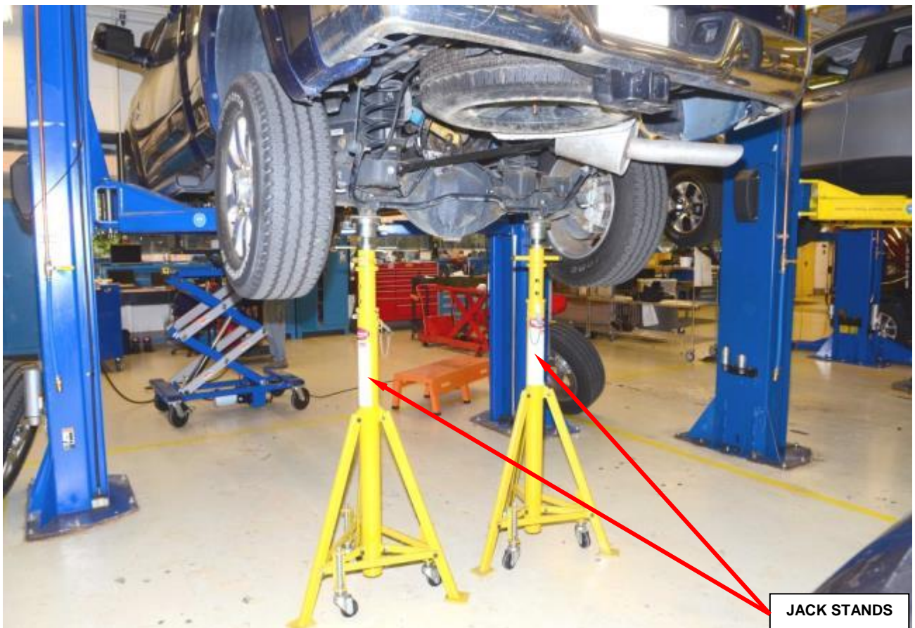
Figure 41 – Secure Vehicle on Hoist with Jack Stands
