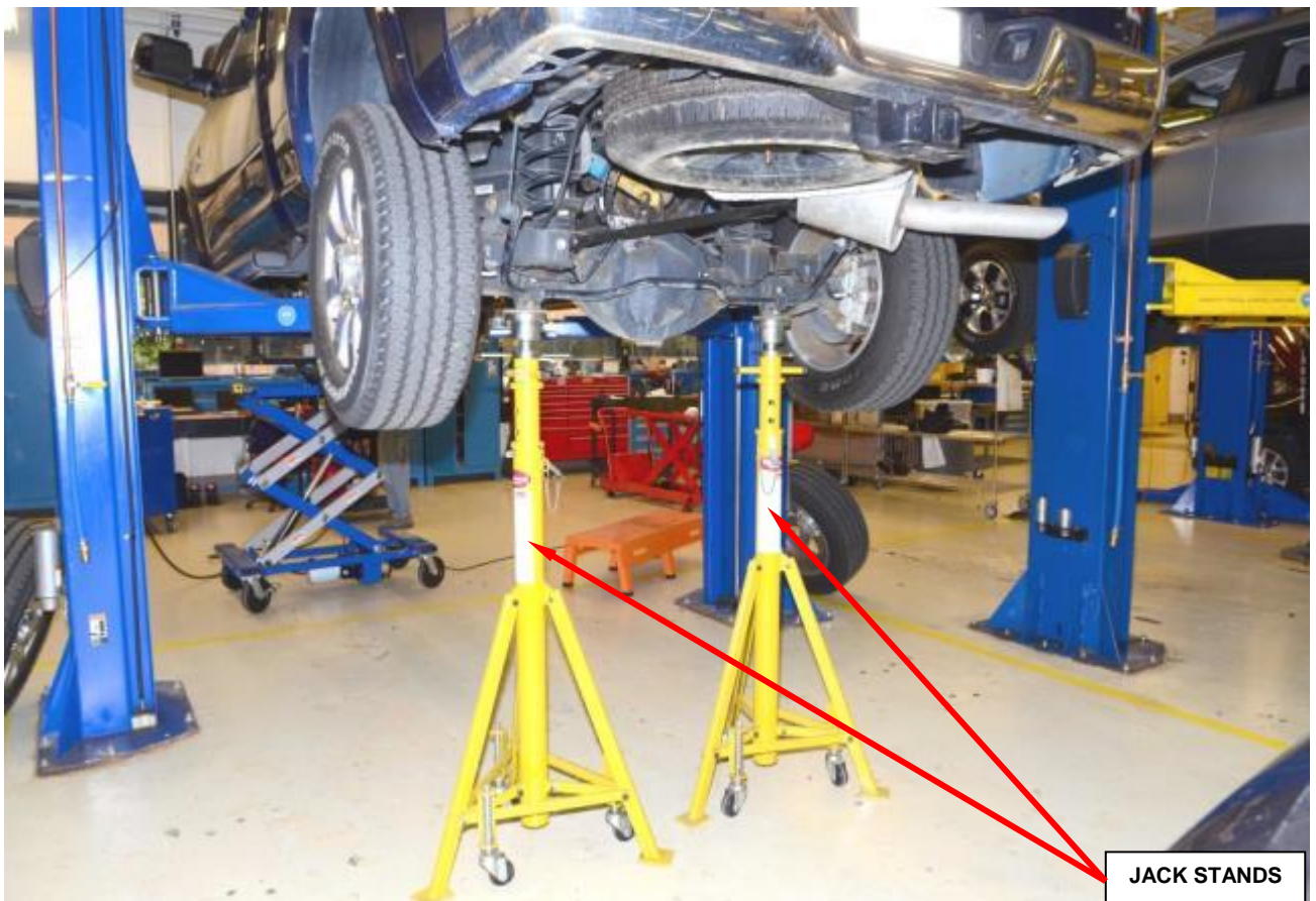
Figure 36 – Secure Vehicle on Hoist with Jack Stands
