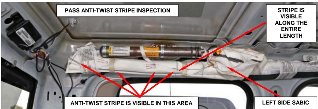
**Figure 21 - Passed Inspection: Anti-Twist Stripe Position
