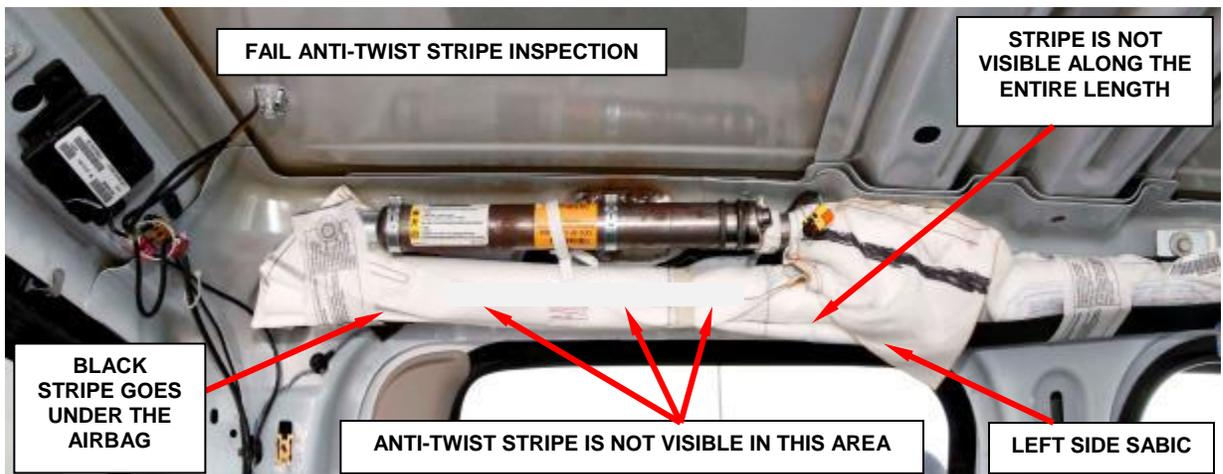
**Figure 23 - Failed Inspection: Anti-Twist Stripe Position
