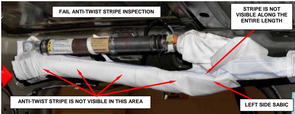
**Figure 22 - Failed Inspection: Anti-Twist Stripe Position
