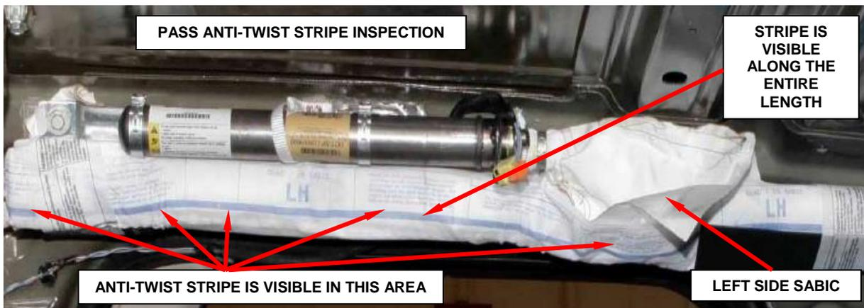
**Figure 20 - Passed Inspection: Anti-Twist Stripe Position
