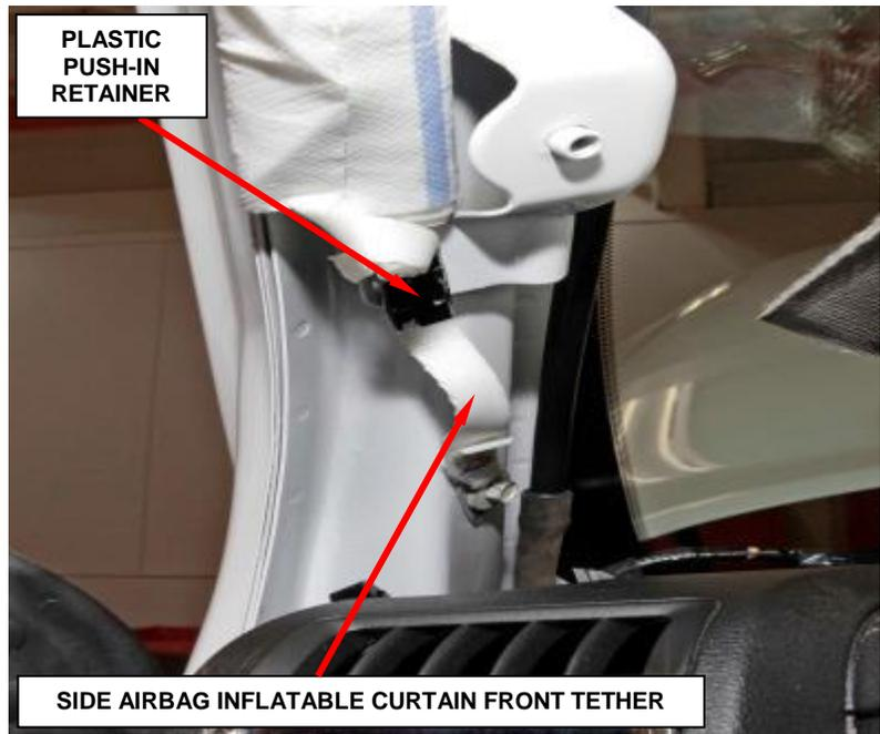
**Figure 28 – Plastic Push-in Retainers**
