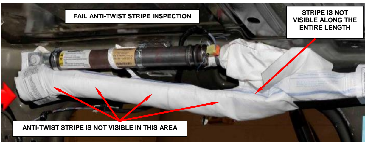
Figure 21 – Failed Inspection: Anti-Twist Stripe Position
