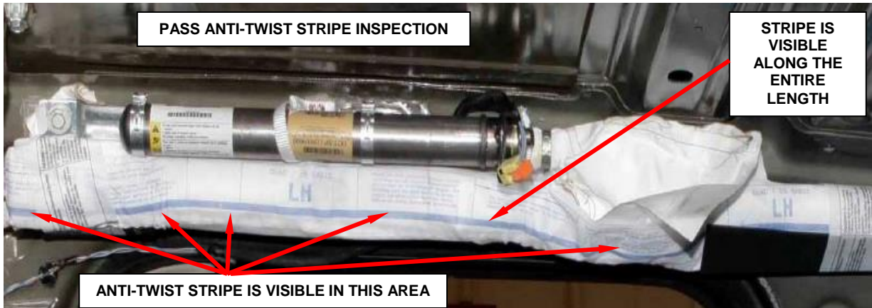
Figure 20 – Passed Inspection: Anti-Twist Stripe Position
