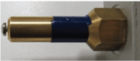
Figure 16: Insert the pressure simulator into the inlet of the PRD block for testing.
