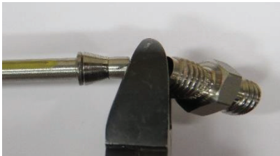
Figure 35: Wire from the LT102B being cut at the pin receiver.
