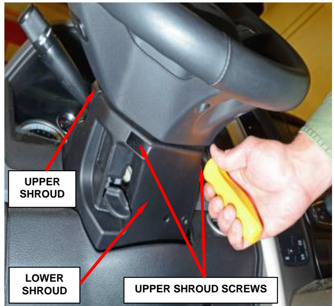
Figure 1 – Upper Shroud Screw Locations
