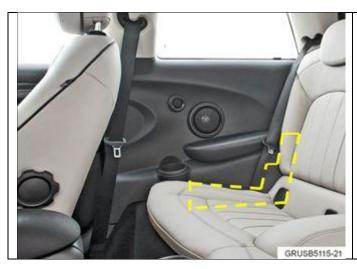
Install a molded structural foam pad to both the left and right rear side trim panels.
