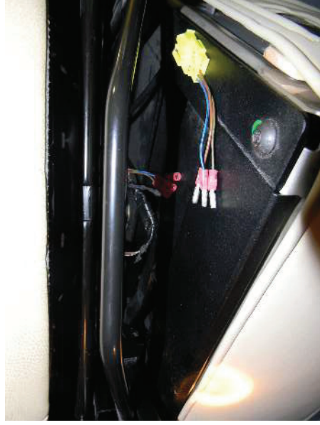
Disconnect bullet connectors
