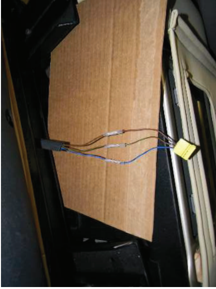
Install heat shrink butt connectors
