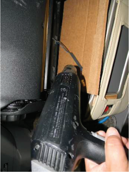
Slide the large heat shrink tubing in place over the butt connectors and shrink
