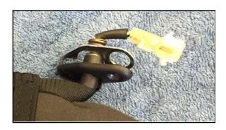
b. Place the tether strap's reinforcement bracket (silver finish) over the sun visor's mirror light harness connector (if equipped) and onto the sun visor's mounting bracket.
