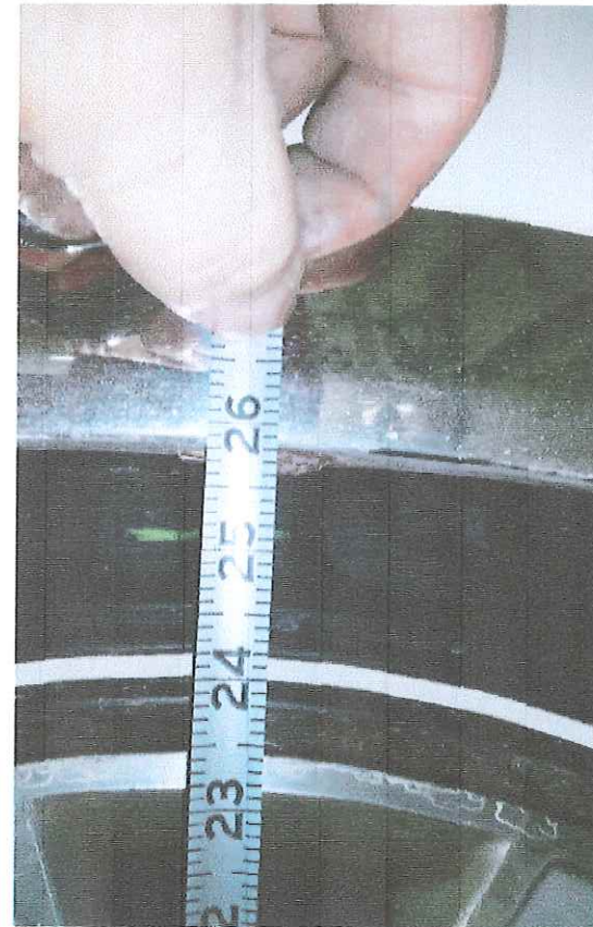
This is with OEM snubber, Approx 25.625".
