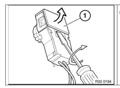
Unlocking the airbag plug connection:
