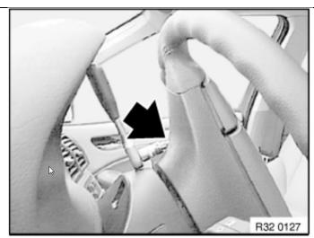
Release screws on both sides (Torx socket T30).
