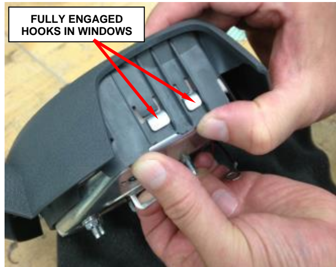
Figure 11 – Inflator Assembly Hooks
