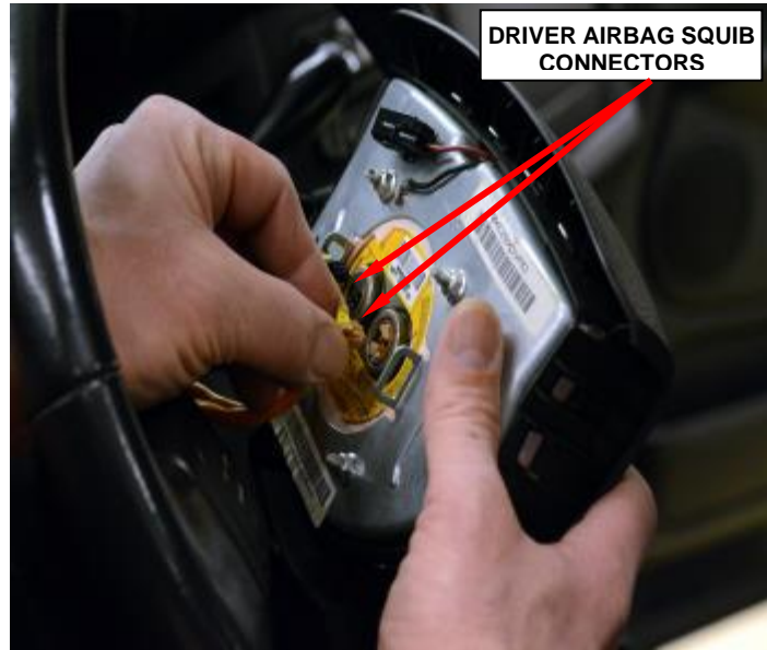
Figure 3 – Driver Airbag Squib Connectors
