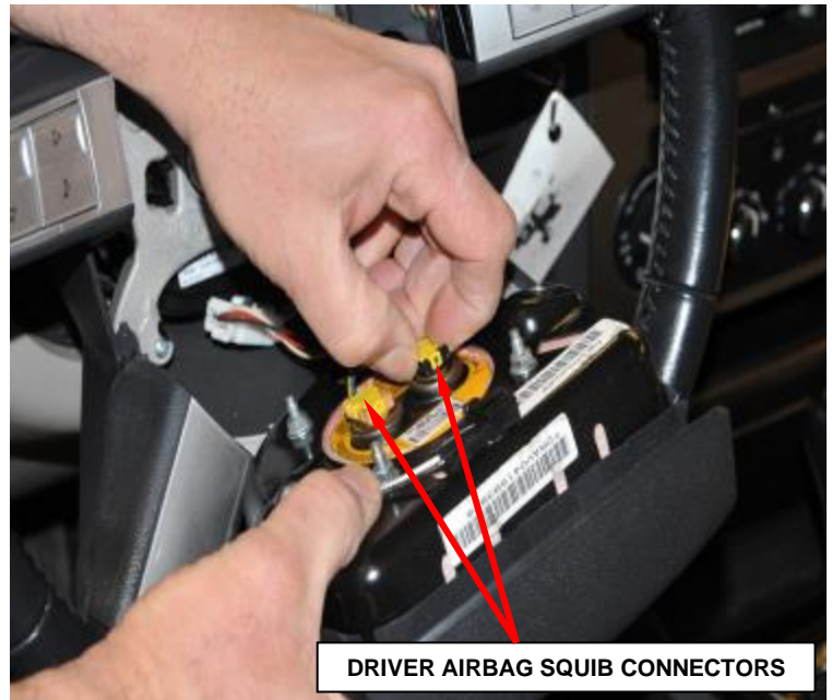
Figure 17 – Airbag Squib Connectors
