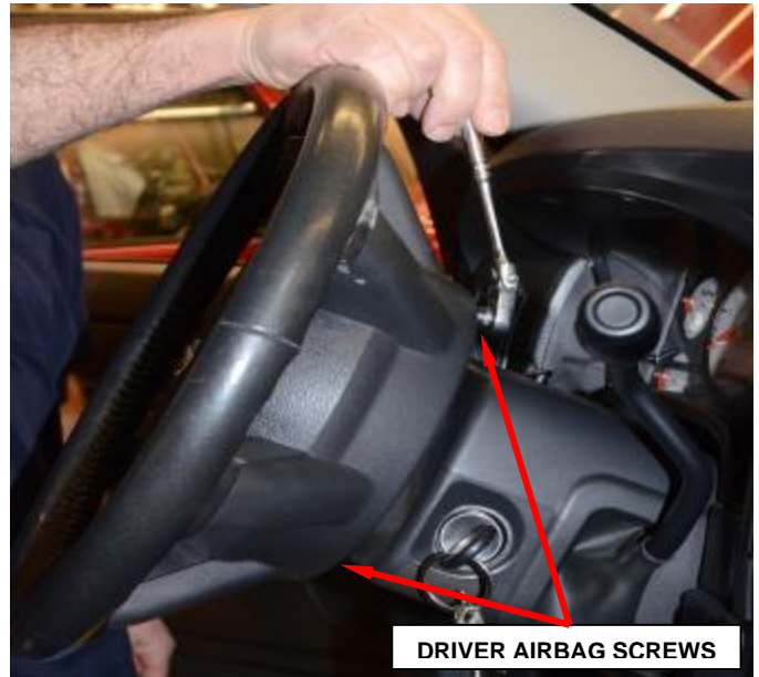
Figure 1 - Driver Airbag Screw Location
