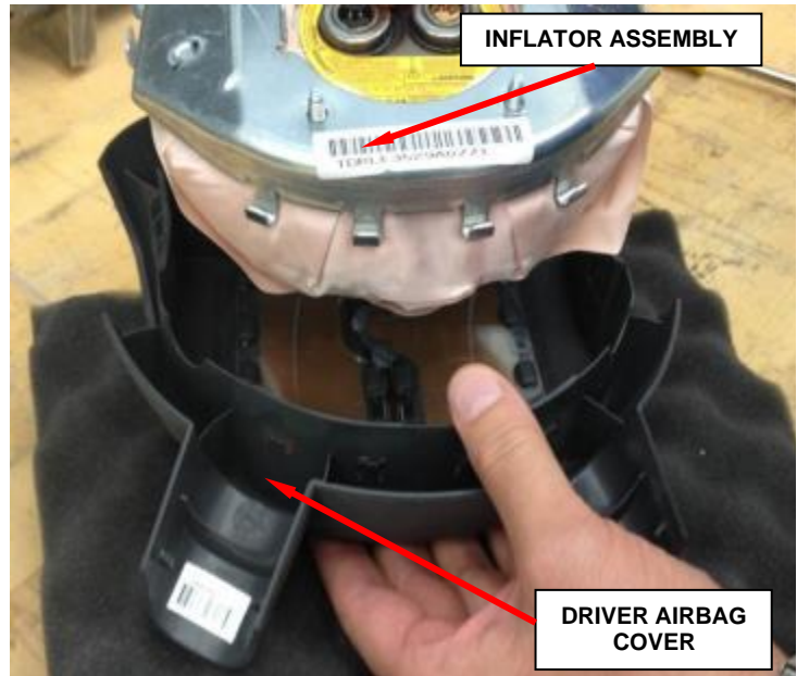
Figure 9 - Inflator Assembly to Driver Airbag Cover
