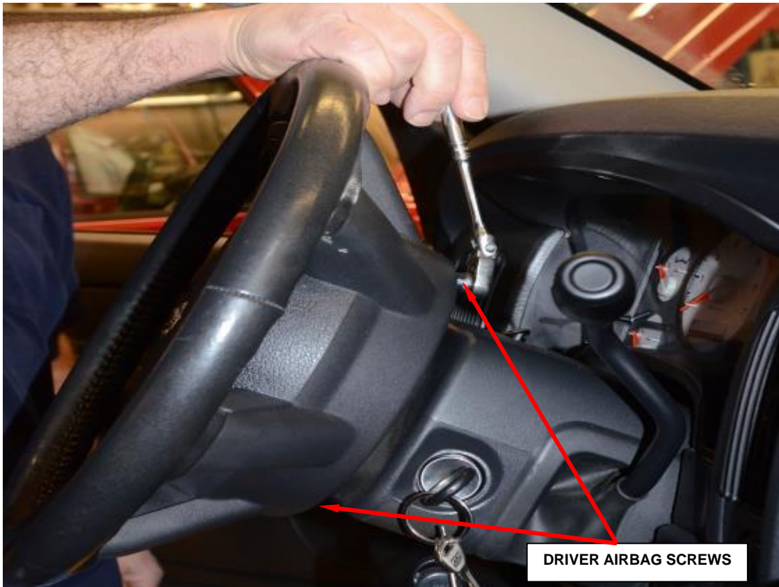
Figure 15 – Typical Driver Airbag Screw Locations
