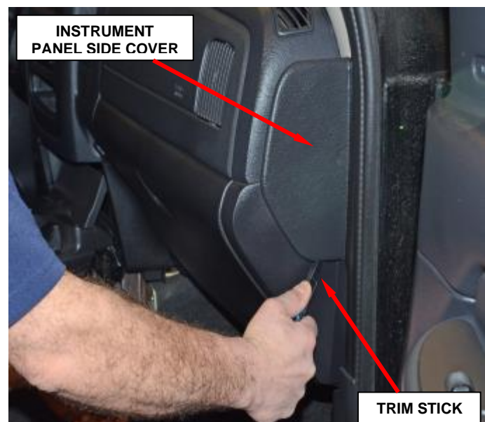
Figure 1 – Instrument Panel Side Cover
