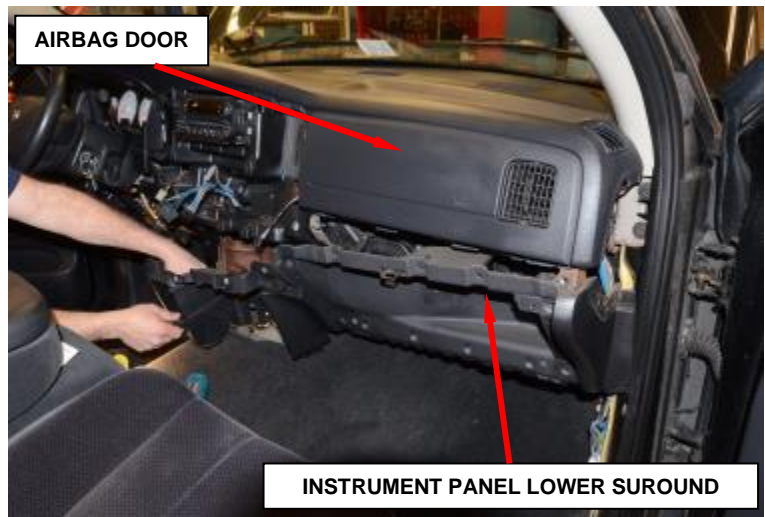
Figure 11 – Instrument Panel Lower Surround
