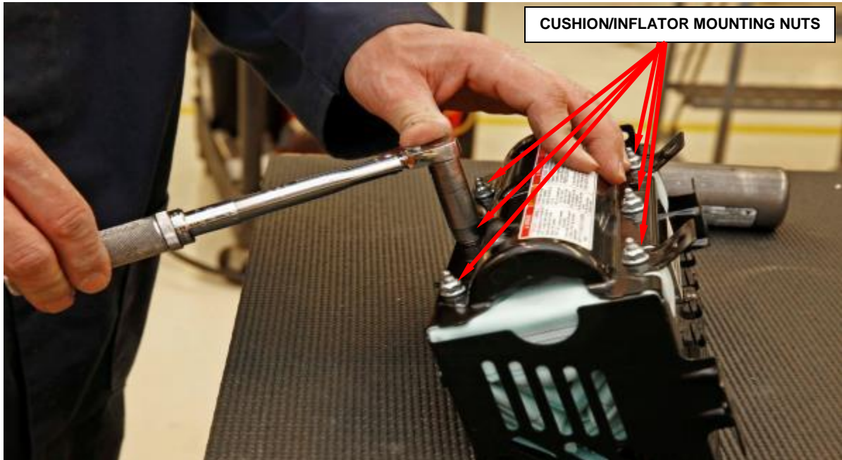
Figure 25 – Cushion/Inflator Assembly Mounting Nuts
