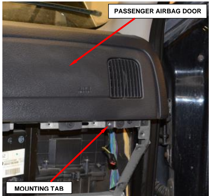
Figure 13 – Panel Outlet Housing Mounting Tab
