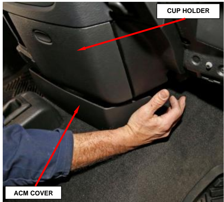
Figure 7 – Airbag Control Module (ACM) Cover
