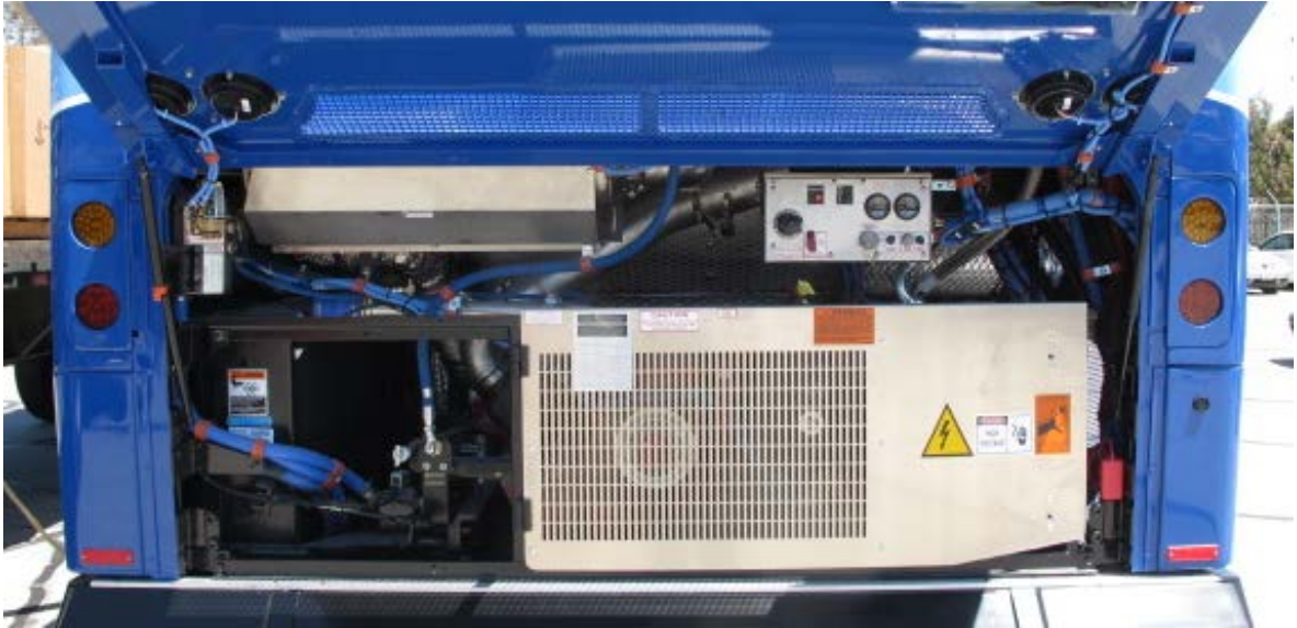
Figure 1: BRT Rear Engine Door Opened
