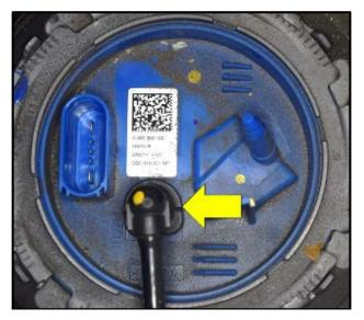
• Disconnect the fuel line <arrow> from the locking flange.
