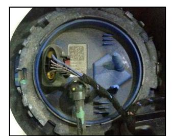
Prior to disassembly, the fuel delivery unit MUST be clean. If excessive dirt or debris is present <as shown>, clean and dry the fuel delivery unit and surrounding areas as necessary.
