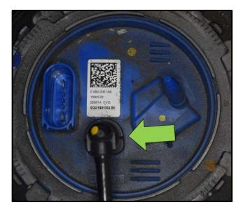
• Attach the fuel line <1> to the locking flange until it clicks into place.
