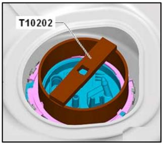
Install the locking ring, and tighten using the Wrench – Fuel Sending Unit – T10202, and torque to 110Nm.
