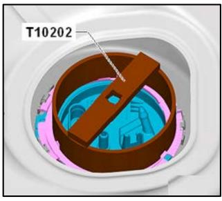
Remove the locking ring using the Wrench
