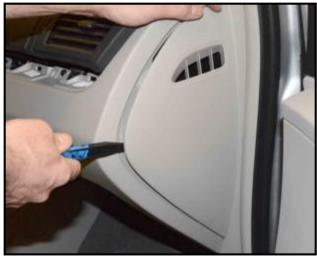
Remove passenger side (right) instrument panel side trim using Trim Removal Wedge –RMCP 101– or equivalent as shown.
