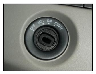
• Reinstall WIN module trim bezel properly into position as shown.
