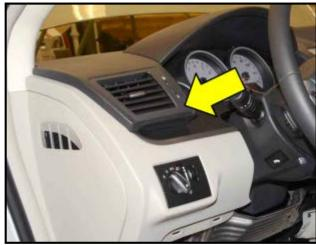
Reinstall the driver side (left) vent <arrow> as shown.
