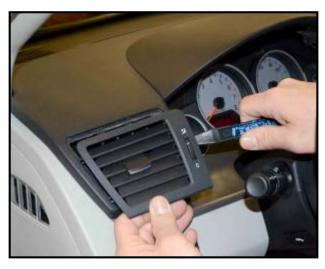
Using Trim Removal Wedge –RMCP 101– or equivalent, loosen and remove the driver side (left) vent trim from the dash as shown.
