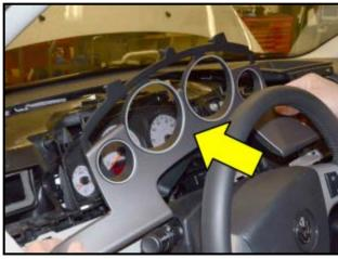
Remove the instrument cluster trim bezel <arrow> as shown.
