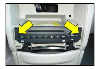
If equipped remove two screws <arrows>, then remove DVD player and disconnect electrical connector.
