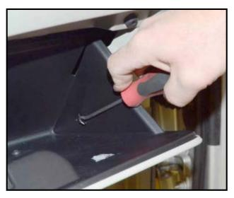
Reposition glove box properly and reconnect glove box return spring using a standard pick tool as shown.
