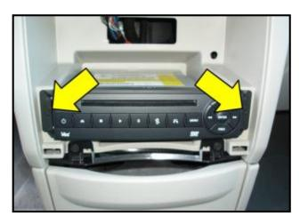
If equipped, reconnect electrical connector for DVD player and reinstall two screws <arrows>.
