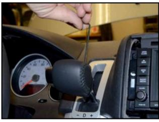
While holding the shift knob button in, reinstall the shift knob onto the shift mechanism shaft and tighten the set screw using a 3mm hex key tool.
