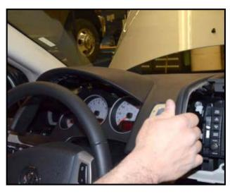
Remove the left instrument panel upper trim panel by gently pulling the panel towards the steering wheel as shown.
