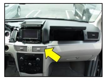
Reinstall the center vent trim assembly <arrow> into the instrument panel as shown.
