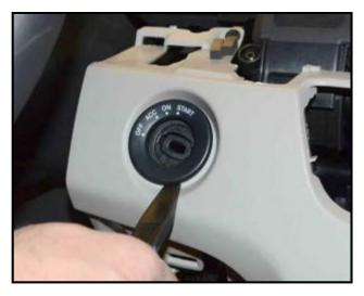
Remove WIN module trim bezel using Trim Removal Wedge –RMCP 101– or equivalent as shown.
