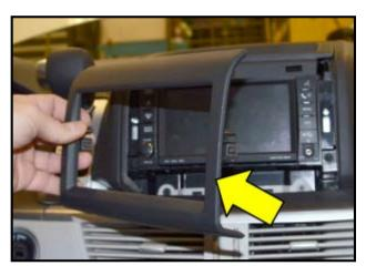
Remove radio trim bezel <arrow> using Trim Removal Wedge –RMCP 101– or equivalent.
