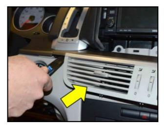
Using Trim Removal Wedge –RMCP 101– or equivalent, loosen the center vent trim assembly <arrow> and remove from instrument panel.
