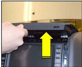
Loosen but do not remove the instrument panel upper storage tray by lifting <in direction of arrow> as shown.
