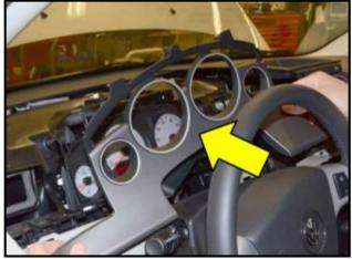
• Reinstall the instrument cluster trim bezel <arrow>.
