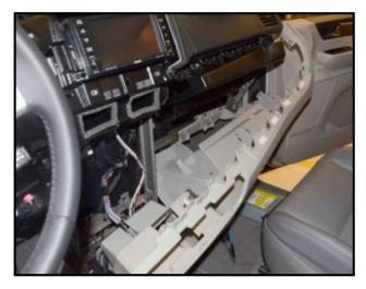
Slightly disengage instrument panel and allow to hang freely.
