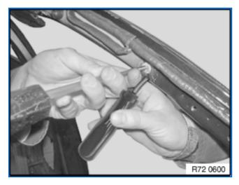
Drive out stem with hammer and 6 mm punch.
