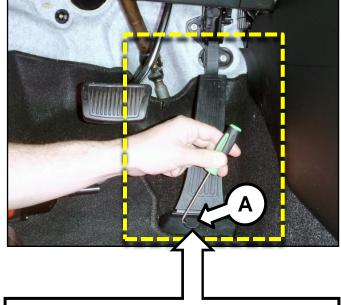
2. Remove one (1) bolt (B) securing the accelerator pedal to the floor pan.
