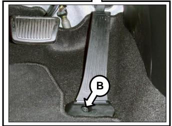
3. Gently rotate the accelerator pedal (C) to the left side, as shown.
