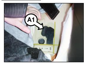
On Soul (PS) vehicles, the rubber pad (P/N 32700B 2110QQK) must align with the side of the pedal mounting bracket, as well as with the raised contour of the floor pan around the rubber plug (A1).
