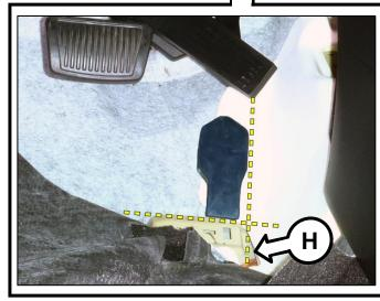
While holding the rubber pad (I) in place, use a permanent marker to transfer the shape of the rubber pad onto the sound deadening material, as shown.
