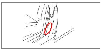
2. LOCATE THE TIRE AND LOADING INFORMATION LABEL ON THE DRIVER-SIDE B-PILLAR (DOOR JAM)
