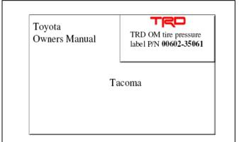
6. INSTALL THE OWNER'S MANUAL LABEL (MDC P/N 00602-35061 ONTO THE UPPER RIGHT FRONT **COVER OF THE OWNER'S MANUAL**
