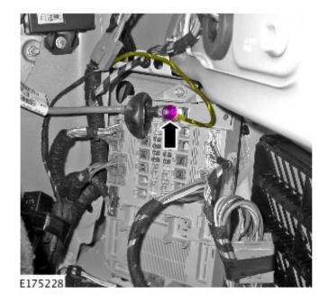
**8.** Using a suitable tape, secure the new link lead and relay harness to the existing harnesses.
