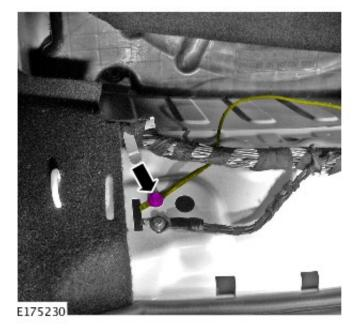
10. CAUTION: Make sure that the ground cable is fully secured in the area of the luggage compartment lid latch, so that the ground cable cannot come in to contact with the latch. Failure to follow this instruction may result in damage to the vehicle.
