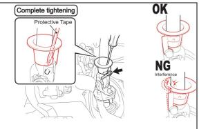
e) Insert a flat tip screw driver wrapped with tape into the gap between the shaft and the thrust stopper as shown while torqueing the intermediate shaft bolt.
