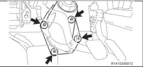
4. REINSTALL THE COLUMN COVER WITH THE 4 CLIPS
