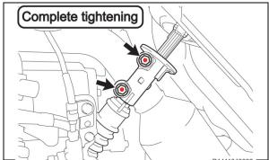
b) Temporarily reinstall the upper bolt.
