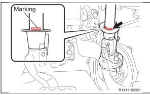
f) Check the mark on the main shaft, to ensure that the intermediate shaft is fully installed on to the main shaft.
