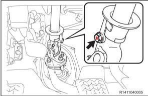
g) Mark the bolt to confirm that it has been properly torqued.
