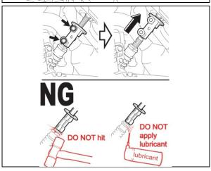
b) Remove the 2 bolts and slide the sliding yoke upward to separarte it from the No. 2 intermediate shaft.
