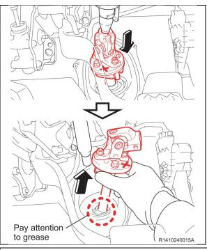
d) Separate the intermediate shaft and steering thrust stopper from the steering column.
