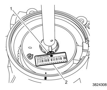
3. Document the last 9 digits of the NEW steering shaft torque sensor on the vehicle repair order. The serial number is located on the bottom of the caution label (2).
