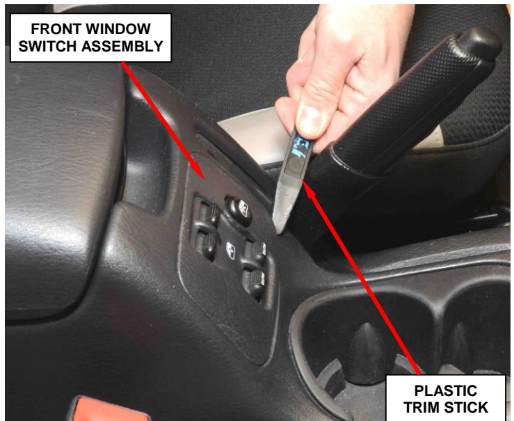
Figure 2 – Front Window Switch Assembly
