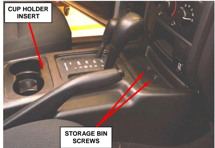
Figure 11 – Storage Bin Screws
