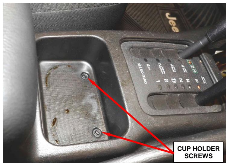
Figure 12 – Cup Holder Screws
