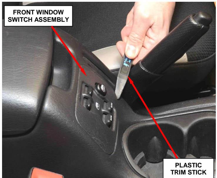
Figure 2 – Front Window Switch Assembly
