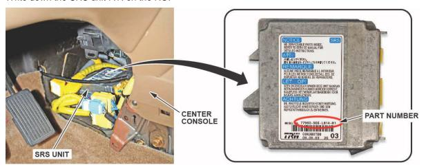
9. Check the SRS unit P/N and arrangement of the subharness against the table below and follow the correct repair action.
