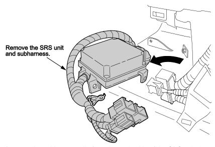
5. Remove the subharness clip from the underside of the SRS unit, then disconnect the subharness from the unit.
