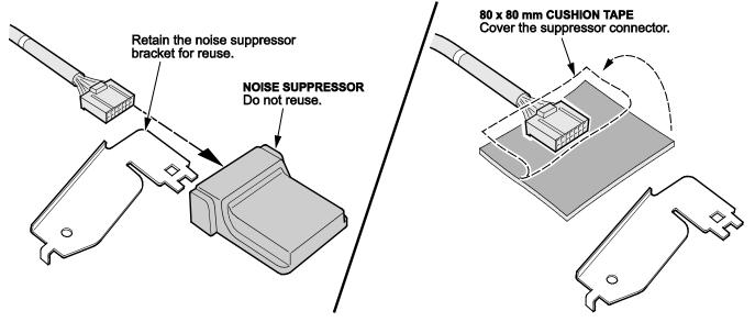
9. Apply a piece of 80 mm x 80 mm cushion tape over the noise suppressor connector as shown.
