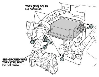
4. Remove the SRS unit by removing the three Torx (T30) mounting bolts.
