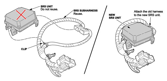
6. Install a new subharness clip onto the original subharness, then connect the subharness to the new SRS unit P/N 77960-S3V-307.
