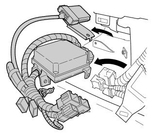
6. Remove the subharness clip from the underside of the SRS unit, then disconnect the subharness from the old SRS unit.
