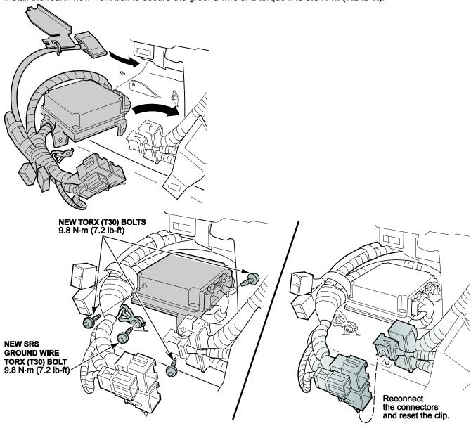
12. Reinstall the bracket using the original bolt as shown. Make sure the connector is pointing downward.
