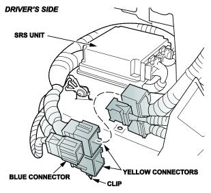
3. Remove the SRS ground wire Torx (T30) bolt.
