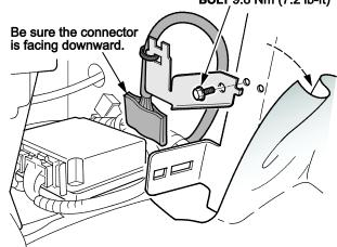
13. Make sure the SRS subharness does not interfere with or rub against the shift cable.
