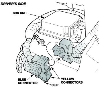
2. Remove the SRS unit by removing the three Torx bolts.
