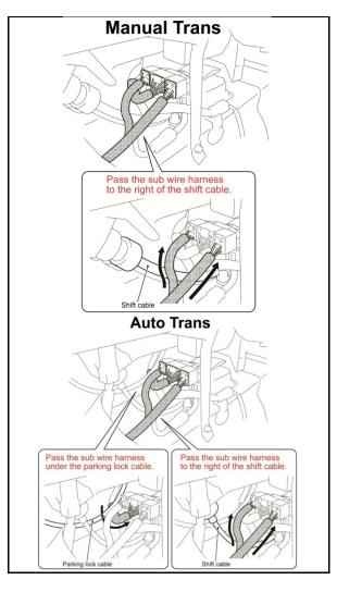
b) Connect the 3 vehicle-side connectors to the **NEW** sub harness. Reference the correct illustration based on transmission type for wire routing.
