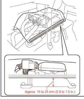
c) Adhere the tape on the sheet to the right side of the airbag sensor approximately 0.6 to 1.0 in. (15 to 25 mm) above the bottom end of the sensor.
