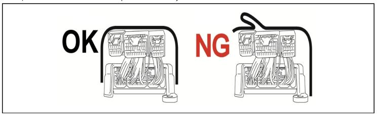
e) Pass a cable tie through the space under the airbag sensor, then connect another cable tie.
