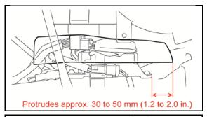
b) Position the sheet so that the edge protrudes 1.2 to 2.0 in. (30 to 50 mm) past the back side of the airbag sensor.
