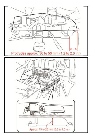
b) Position the sheet so that the edge protrudes 1.2 to 2.0 in.(30 to 50 mm) past the back side of the airbag sensor.
