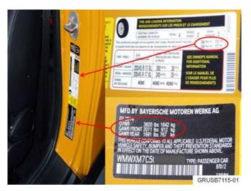
The maximum vehicle load (on the tire label) and gross vehicle weight rating (GVWR, on the VIN label) have been increased.
