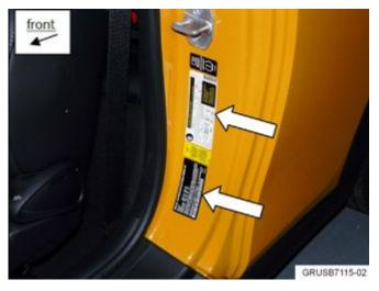
Compare the new label versus the old label to verify that the VINs match and the GVWR is different (has increased) **before the old label is removed!**
