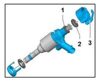
Ü Using the appropriate seals from injector seal kit, P/N 06J998907B, replace the upper seals <1 and 2> and the metal retainer <3> on each fuel injector.
