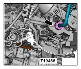
Ü Loosen the union nut on the fuel rail <arrow> with the Flare Nut Attachment 17mm – T10456 and remove the high pressure line <as shown>.
