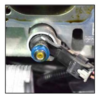
Ü Lubricate the upper o-ring on each fuel injector with clean engine oil <as shown>.
