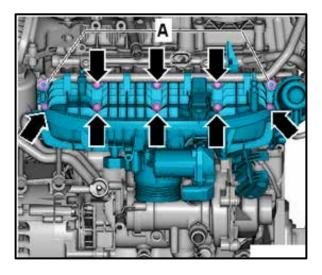
Ü Remove the mounting nuts <A> and the mounting bolts <arrows> from the intake manifold.
