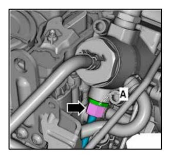
Ü Using an appropriate torque wrench and crow's foot fitting, torque the flare nut <arrow> onto the high pressure pump adapter at 27Nm.
