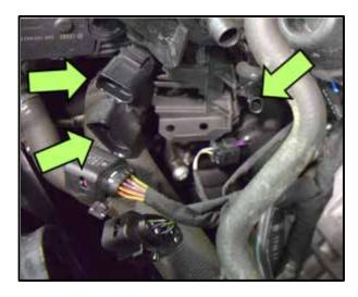
Ü Disconnect the wiring harness connectors <arrows> underneath the intake manifold.
