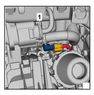
Ü Disconnect the Camshaft Position Sensor G40 connector <1>.
