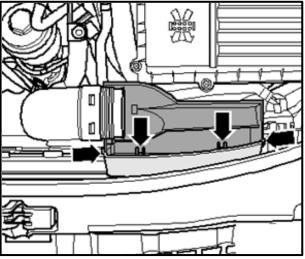
Ü Release the clips <arrows> and unfasten the lower air guide.
