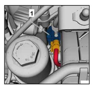
Ü Disconnect the IMRC position sensor G336 <1>.
