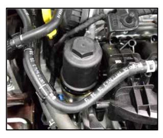
· Loosen and remove the oil filter.
