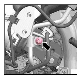
Remove the screw <arrow> from the mounting clamp.
