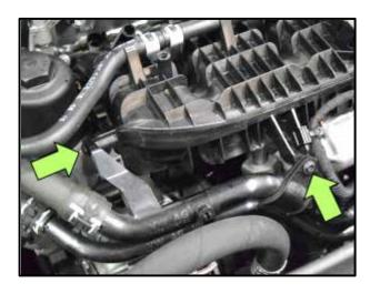
Ü Reinstall the coolant hose mounting bolts <arrows>.
