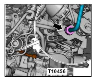
Ü Using an appropriate torque wrench and the flare nut attachment T10456 <as shown>, torque the flare nut onto the fuel rail adapter at 27Nm.
