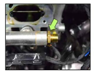
Install the new fuel line adapter <arrow>, P/N 06K127065B, into the end of the fuel rail and torque to 40Nm.
