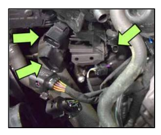
Ü Reconnect the wiring harness connectors <arrows> underneath the intake manifold.
