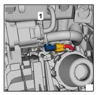
$\ddot{\text{U}}$  Reconnect the camshaft position sensor G40 <1>.
