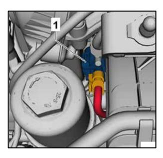
Ü Reconnect the IMRC position sensor G336 <1>.
