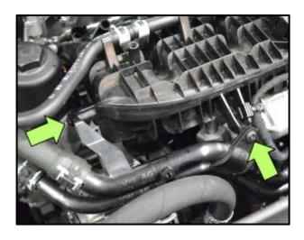
Reinstall the coolant hose mounting bolts <arrows>.
