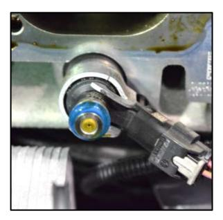
← Lubricate the upper o-ring on each fuel injector with clean engine oil <as shown>.
