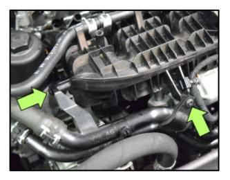
Remove the mounting bolts <arrows> for the coolant line from the intake manifold.
