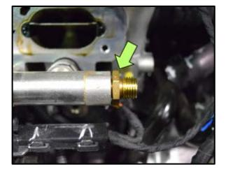
Note: It is not necessary to apply any sealant to the fuel rail, lines, or other fuel system fittings during this repair.
