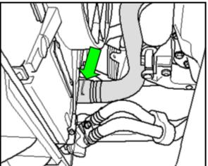
← If the drain plug is not present, disconnect the right lower radiator hose and allow the coolant to drain.
