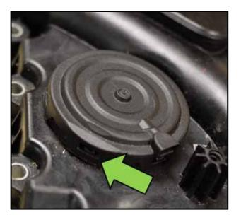
• Install the spring, diaphragm, and breather cap onto the crankcase breather.
