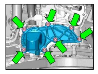
Tip: Coat the new O-rings and gaskets for the coolant system with clean coolant prior to installation.
