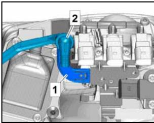
Free up the brake booster vacuum hose <2> on the bracket <1>.
