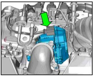
Disconnect the control module (J808) <arrow>.
