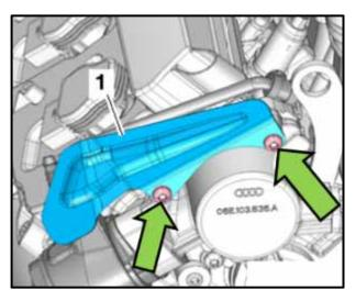
Remove the mounting screws <arrows> and the protective plate <1>.
