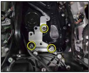
Remove the retaining screws <circles> and mounting bracket from the top of the crankcase breather.
