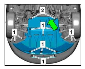
Raise vehicle on hoist and reinstall the noise insulation and the mounting parts <1, 2, arrow>.
