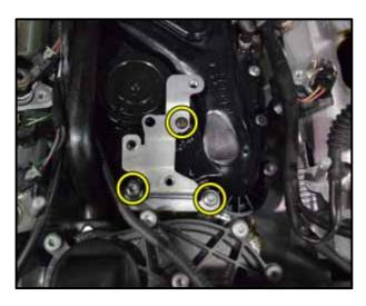
Reinstall the bracket and retaining screws <circles> onto the crankcase breather.
