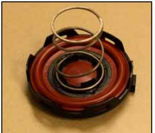
Assemble the replacement cap, diaphragm, and spring as shown.
