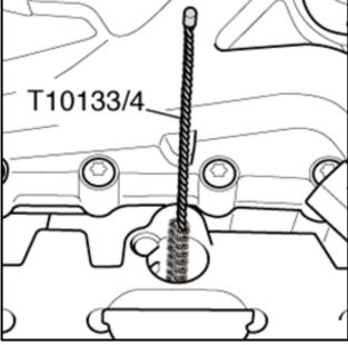
← Clean the fuel injector hole inside the cylinder head with the nylon cylinder brush T10133/4 <as shown>.
