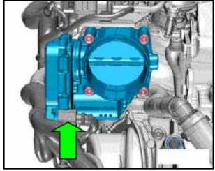
Disconnect the throttle valve control module J338 <arrow>.
