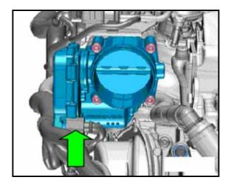
Reconnect the connector <arrow> on the throttle valve control module J338.
