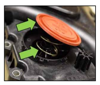
Remove the diaphragm and spring from the crankcase breather as shown <arrows>.
