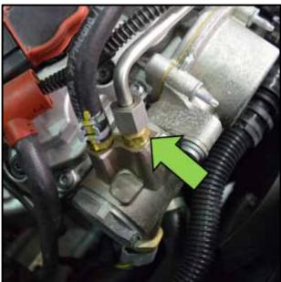
Wrap a clean cloth around the fuel line threaded connection <arrow> and open it slowly, allowing residual fuel pressure to escape. Once the fuel pressure is relieved, fully remove the threaded connection.
