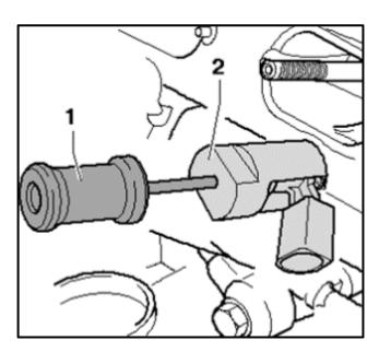
If the fuel injector does not fit into the head by pressing gently, use the puller – T10133B/2A <2> with the Sliding Hammer T10133A/3 <1> to guide the fuel injector into place.
