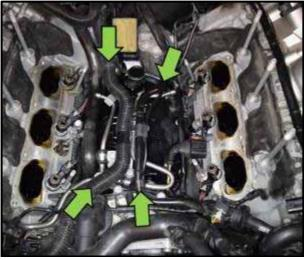
Position the plastic lines back to their original routing <arrows> and reconnect them as necessary.
