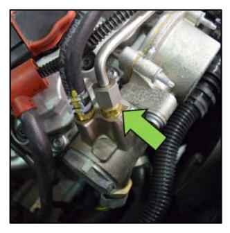
Torque the threaded connection to 27Nm.
