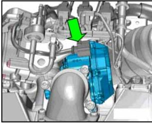
Reconnect the connector <arrow> on the control module J808.
