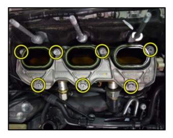
Remove the mounting fasteners <circles> from the intake manifold/fuel rail assembly.
