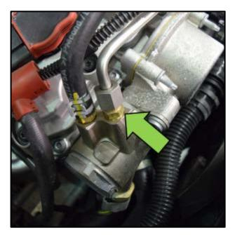
Torque the threaded connection to 27Nm.
