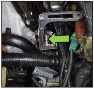
Reinstall the mounting bracket and screws <arrow>.
