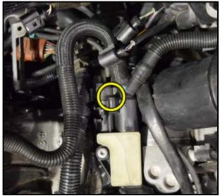
Reinstall the crankcase breather hose onto the back of the crankcase breather and reinstall the mounting screw <circle>.
