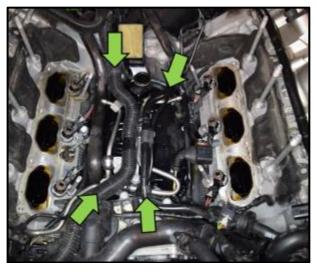
Remove the mounting screws <circles> and mounting bracket from the top of the crankcase breather.
