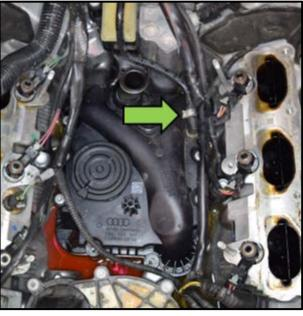
Reinstall the hose and an appropriate claim <arrow> onto the crankcase breather.
