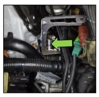
Remove the mounting screws <arrow> from the mounting bracket.
