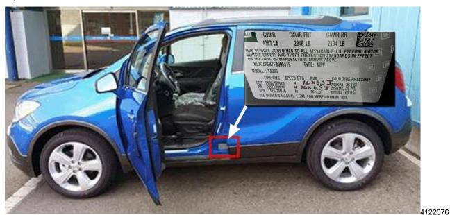
Locate the Vehicle Certification Label on the lower section of the driver's door jamb as illustrated above.
