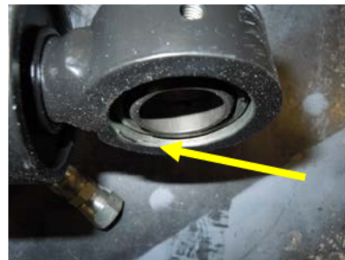
Rod end - recessed .13 inch each side
