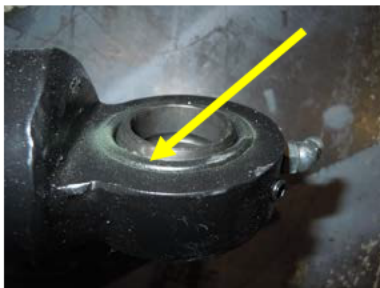
Base end - bearing outer race flush
