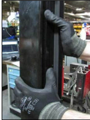
Figure 6, Pushing Handle-Side Window Frame Against the Bus Structure
