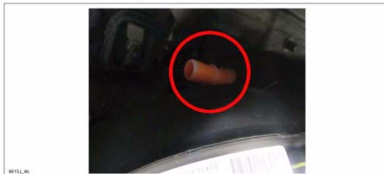
9. Install the test device.
