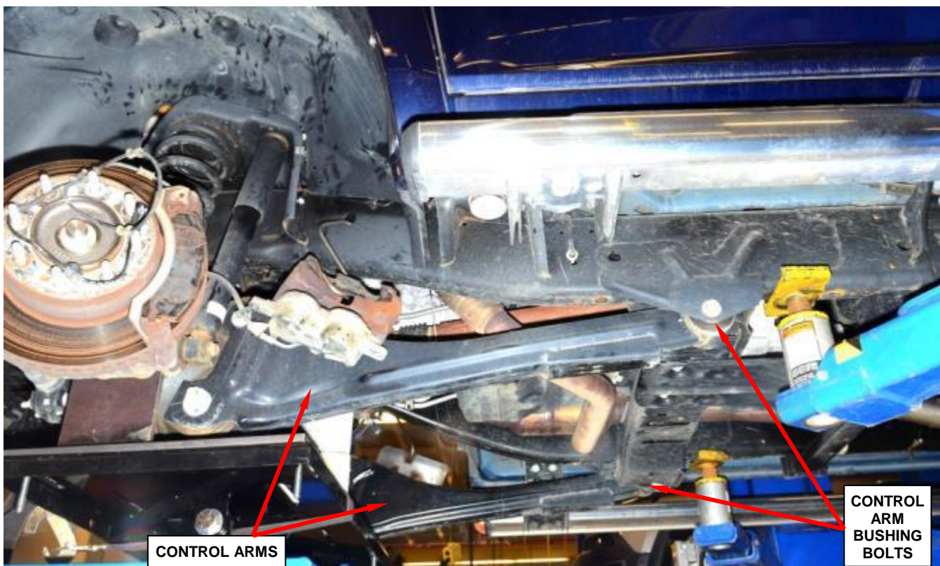
Figure 39 – Control Arm Bushing Bolts
