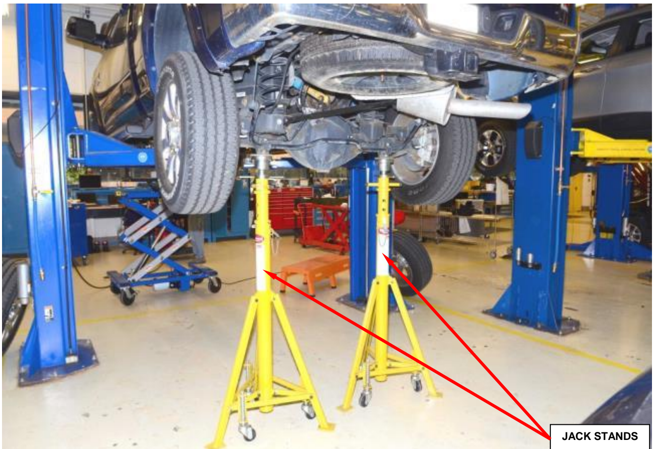
Figure 35 – Secure Vehicle on Hoist with Jack Stands
