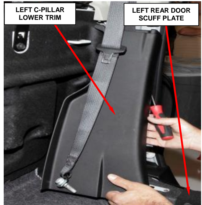
Figure 8 – Left Lower C-Pillar Trim
