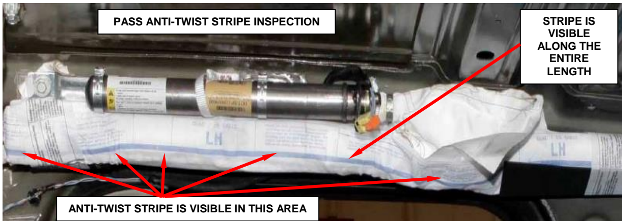
Figure 20 – Passed Inspection: Anti-Twist Stripe Position
