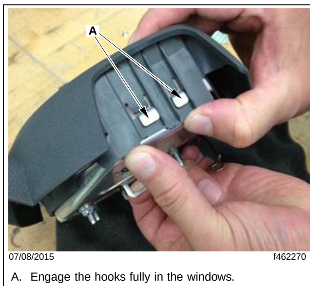
Fig. 7, Inflator Assembly Hooks
