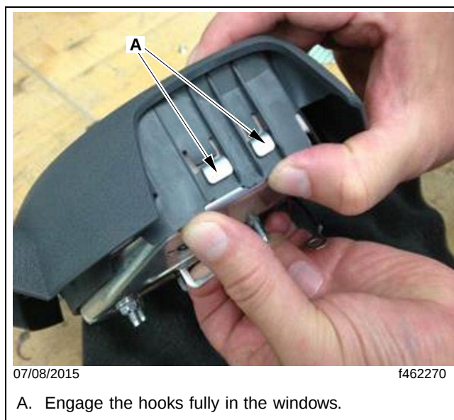
Fig. 7, Inflator Assembly Hooks
