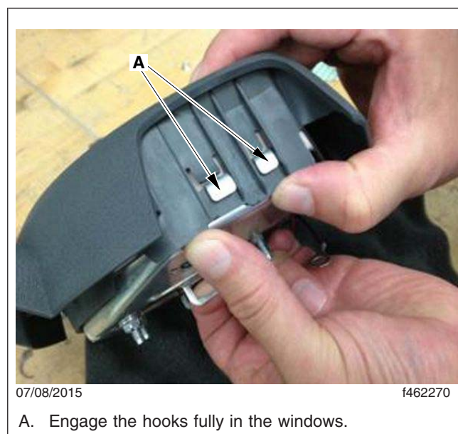
Fig. 7, Inflator Assembly Hooks
