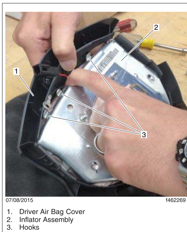
Fig. 6, Removing the Inflator Assembly
